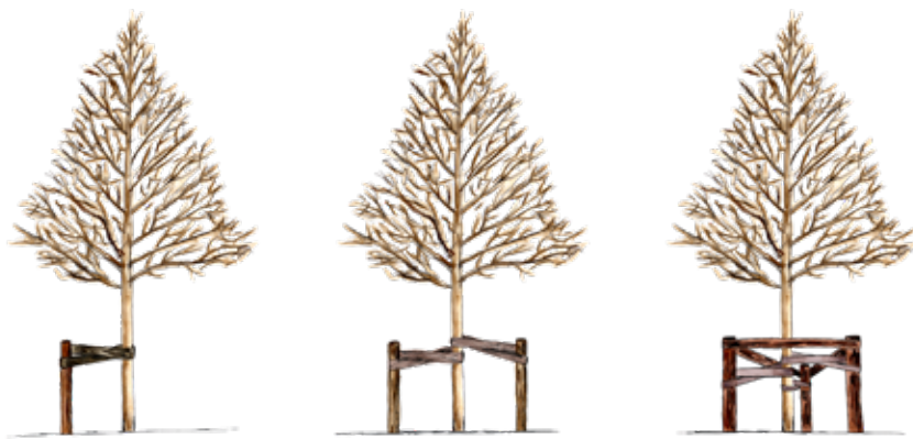
Anchoring above the ground using one, two or three stakes
